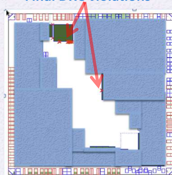
Final DRC violations
